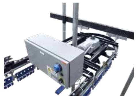
Direct drive motor with soft start feature.
